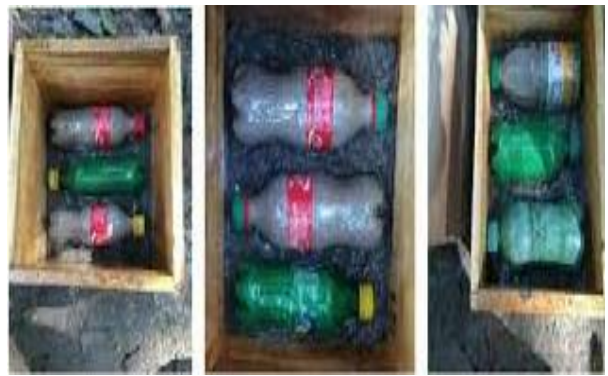
Fig 2: Layer of bottles placed in brick
